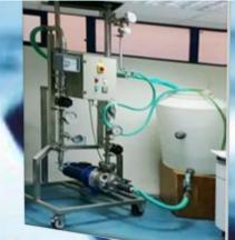
UF device: ceramic, length: 1020mm, pore size: 100nm, surface area: 0.24m²
